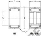
Heavy duty needle roller bearings
